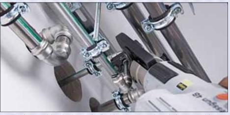
The best tool for the Antarctic: Problem-free pressing of pipes at ambient temperatures around freezing and in the tightest of spaces – with the help of press rings. (Photo: Viega)
